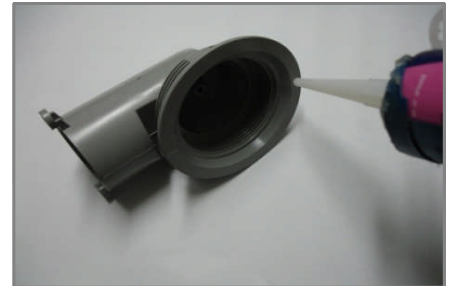
Apply an adequate amount of silicone to front flange of body
