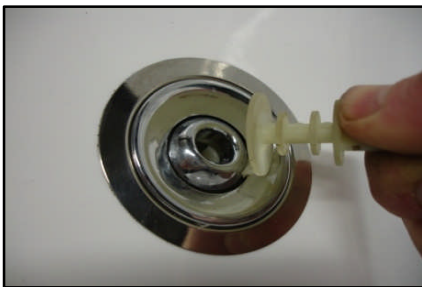
Using Service Tool MT0268, push eyeball back and clip tool under edge of jet face.
