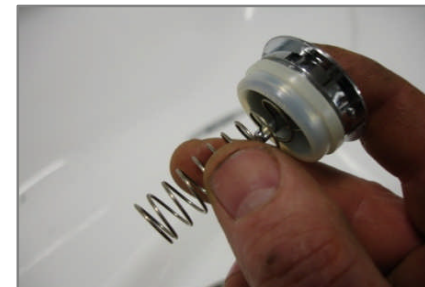
Remove trim and plunger, allowing access to bellows and spring.
